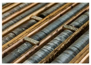
**Core drilling sample**
